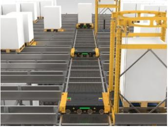
The iCUBE system uses an array of energy-efficient E-Carriers and Lifts, ensuring redundant operation while allowing parallel fulfillment of inbound, outbound, and order picking processes.
