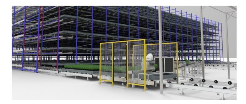
The proven LOGIQS rolling bench design further contributes to the flexibility and durability of the Greencube system. The Ebb and flood benches can be configured a large diversity of crops.
